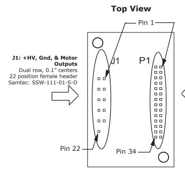
**Drive viewed from above looking down on the pc board on which it is mounted.** Pins shown in grey are unused locations in PC board socket
